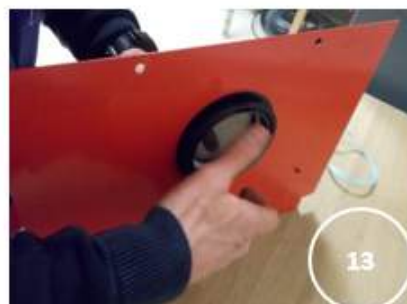
Then, put the nut on the thread and tighten with hand.
