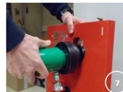
Connect the pump to the piston.
