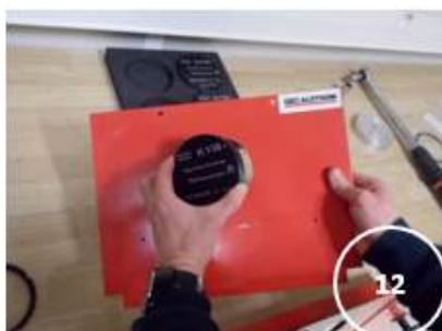
Put the window in the drilling, engraved cover on the outer side of the cell.
