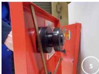
Mount the cup shape drilling tool and counter cup shape on both sides of the sheet metal on axis \varnothing 28 mm.
