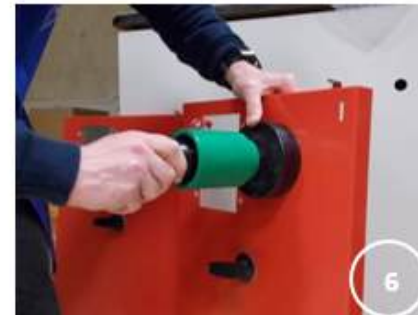
Screw axi \varnothing 28 mm on the piston.
