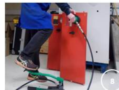
Operate the pump to cut the sheet metal.
